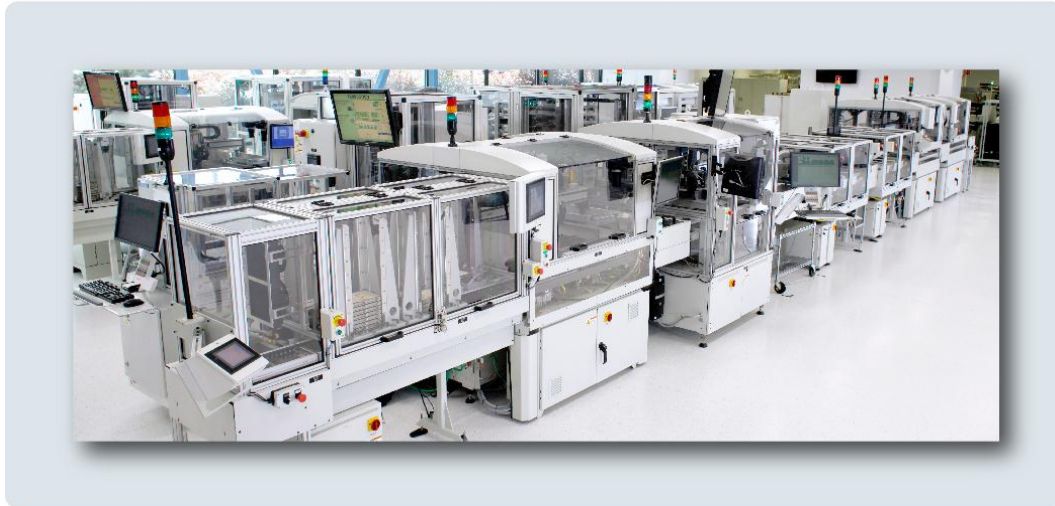
Figure 10. The AFTS handles all module functional tests during production
