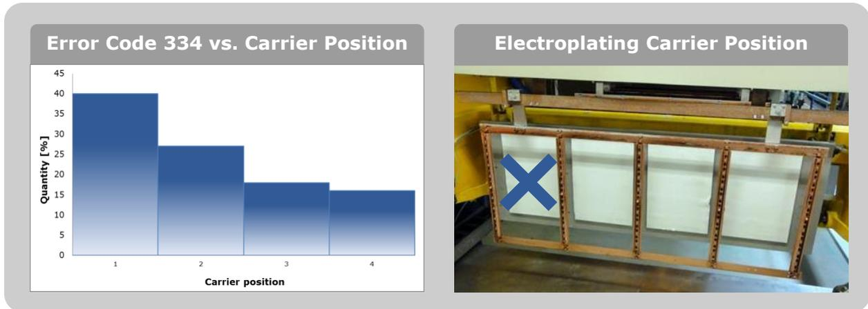
Figure 4. Combining error codes with product related data shows a correlation to the position within the electroplating carrier
