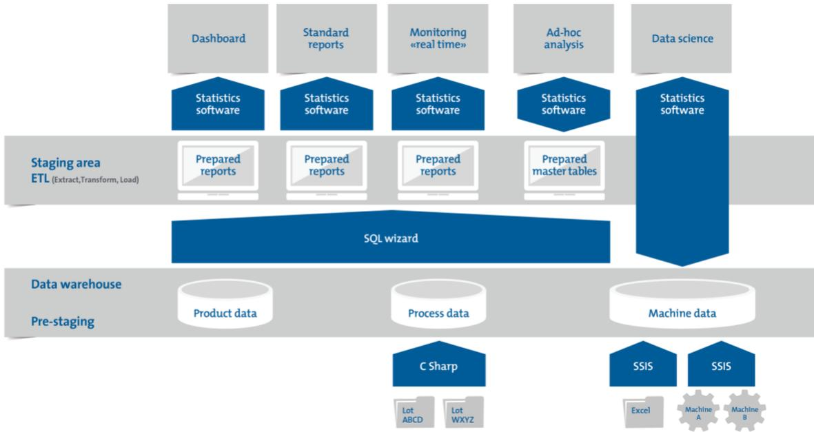
Figure 2. Two-stage DYCO IC2 approach to data processing
